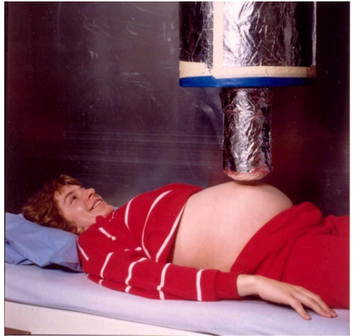
Recording fetal magnetocardiogram in the magnetically shielded room.
